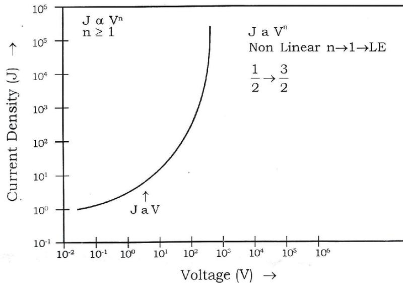
Fig. 2. SCL Current-voltage characteristic of an insulator with traps lying below the fermi level
