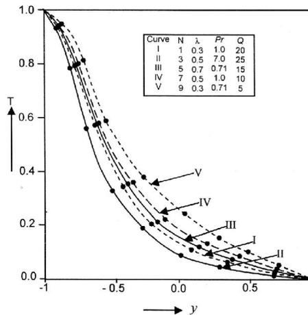
Fig. 3. The temperature distribution versus  $y$  for different values of  $N, \lambda, Pr$  and  $Q$  ( $M=0.5, K_0=0.3, \alpha'=1, Sc=0.40, K_1=1$ ).
