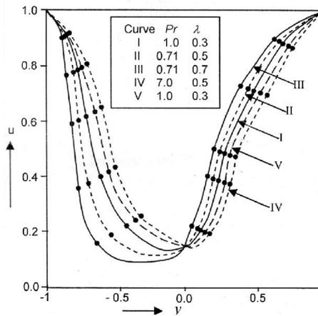
Fig. 2. The velocity distribution versus  $y$  for different values of  $Pr$  and  $\lambda$  ( $M=0.5, N=1, \alpha'=1, Sc=0.40, K_1=1, K_0=0.3, Q=5$ ).
