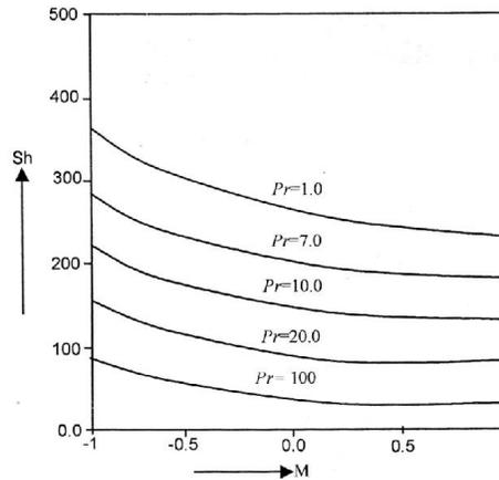
Fig. 7. Sherwood number versus  $M$  for different value of  $Pr$  ( $N = 1, K_0 = 0.3, \alpha' = 1, Sc = 0.40, K_1 = 1, \lambda = 0.3, Q = 5$ )
