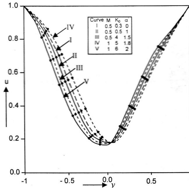
Fig. 1. The velocity distribution versus  $y$  for different values of  $M$ ,  $K_0$  and  $\alpha'$  ( $N = 1, Pr = 7.0, \lambda = 0.3, Sc = 0.40, K_1 = 1, Q = 5$ ).
