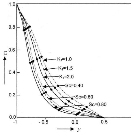
Fig. 4. The concentration distribution versus  $y$  for different values of  $K_1$  and  $Sc$  ( $M = 0.5, Pr = 7, \lambda = 0.3, N = 1, \alpha' = 1, K_0 = 0.3, Q = 5$ ).
