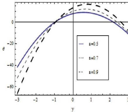
Fig. 12. The variation of  $\theta$  with  $y$  for different values of  $a$  at  $b = 0.5; d = 1; Q = 0.5; E_c = 0.2; Pr = 0.2; \alpha = 0.3; \phi = \pi/2$ ;
