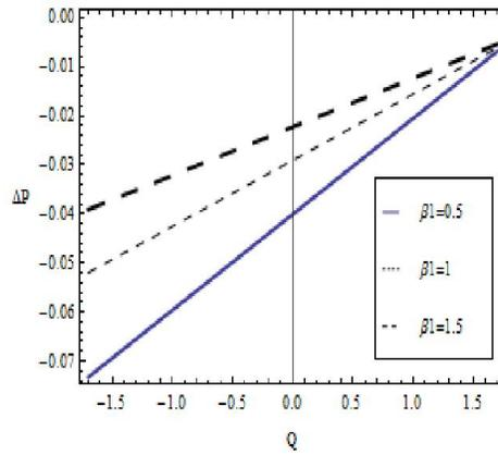
Fig. 7. The variation of  $\Delta p$  Vs  $Q$  for different values of  $\beta_1$  at  $a = b = 0.5$ ;  $b = \alpha = 0.3$ ;  $d = 1$ ;  $\phi = \pi/2$ ;
