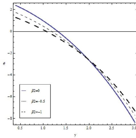
Fig. 14. The variation of  $\theta$  with  $y$  for different values of  $\beta_2$  at  $a = b = 0.5; d = 1; Q = 0.5; E_c = 0.2; Pr = 0.2; \alpha = 0.3; \phi = 0;$
