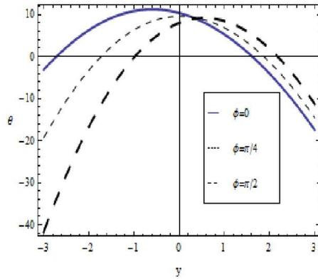
Fig. 13. The variation of  $\theta$  with  $y$  for different values of  $\phi$  at  $a = b = 0.5; d = 1; Q = 0.5; E_c = 0.2; Pr = 0.2; \alpha = 0.3;$
