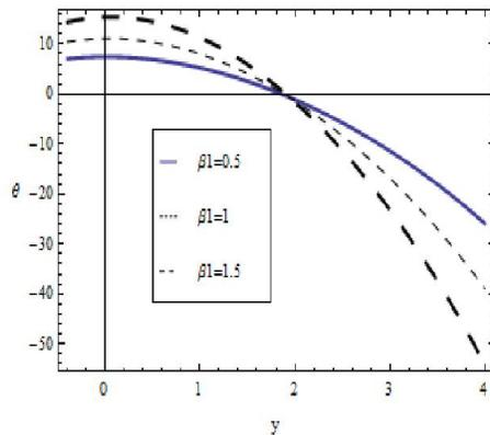
Fig. 15. The variation of  $\theta$  with  $y$  for different values of  $\beta_1$  at  $a = b = 0.5; d = 1; Q = 0.5; E_c = 0.2; Pr = 0.2; \alpha = 0.3; \phi = 0;$
