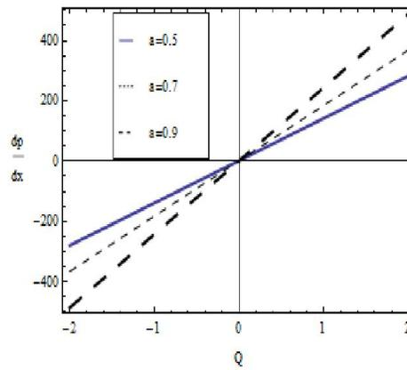
Fig. 8. The variation of  $\frac{dp}{dx}$  with  $Q$  for different values of  $a$  at  $b = 0.5$ ;  $\phi = \pi/2$ ;  $d = 1$ ;
