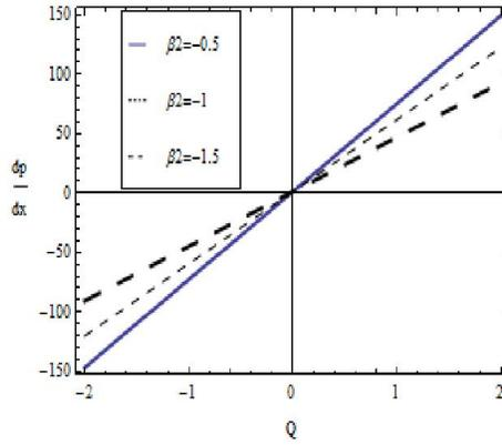
Fig. 10. The variation of  $\frac{dp}{dx}$  with  $Q$  for different values of  $\beta_2$  at  $a = b = 0.5; d = 1; \phi = 0$ ;
