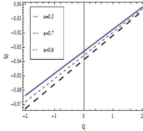
Fig. 4. The variation of  $\Delta p$  Vs  $Q$  for different values of  $a$  at  $b = 0.5$ ;  $\phi = \pi/2$ ;  $\alpha = 0.3$ ;  $d = 1$
