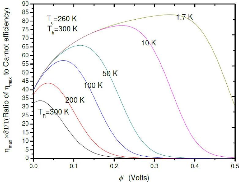
Fig. 2. The ratio of maximum cooling efficiency  $\eta_{\max}$  to Carnot efficiency as a function of barrier height  $\phi'$  at  $T_c = 260$  K and  $T_h = 300$  K for different  $TR$  [K] = 1.7, 10, 50, 100, 200 and 300.
