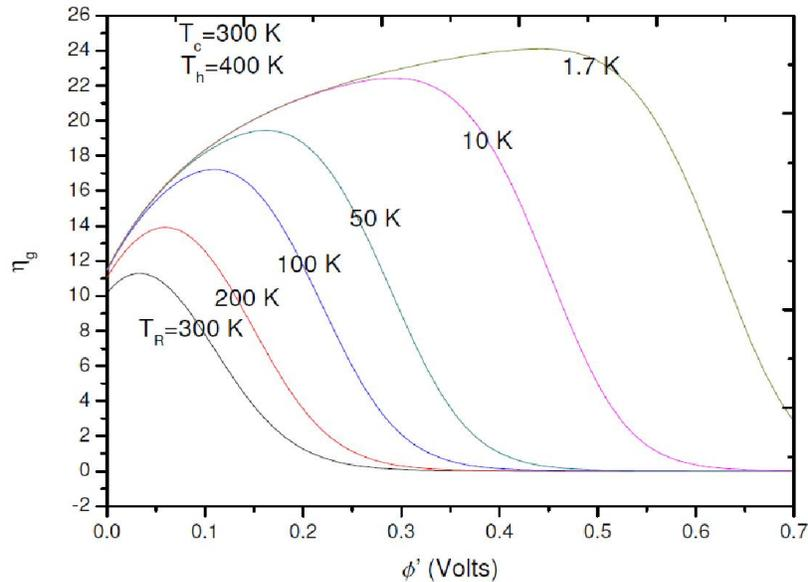
Fig. 3. The efficiency  $\eta_g$  for power generation as a function of barrier height  $\phi'$  at  $T_c = 300 \text{ K}$  and  $T_h = 400 \text{ K}$  for different  $TR [\text{K}] = 1.7, 10, 50, 100, 200,$  and  $300$ .
