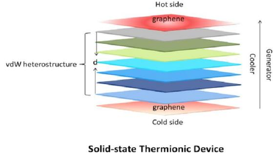
**Fig. 1 : Schematic diagram of van der Waals heterostructure-based solid state thermionic device with graphene electrode. where  $d$  is the thickness of van der Waals heterostructure.**
