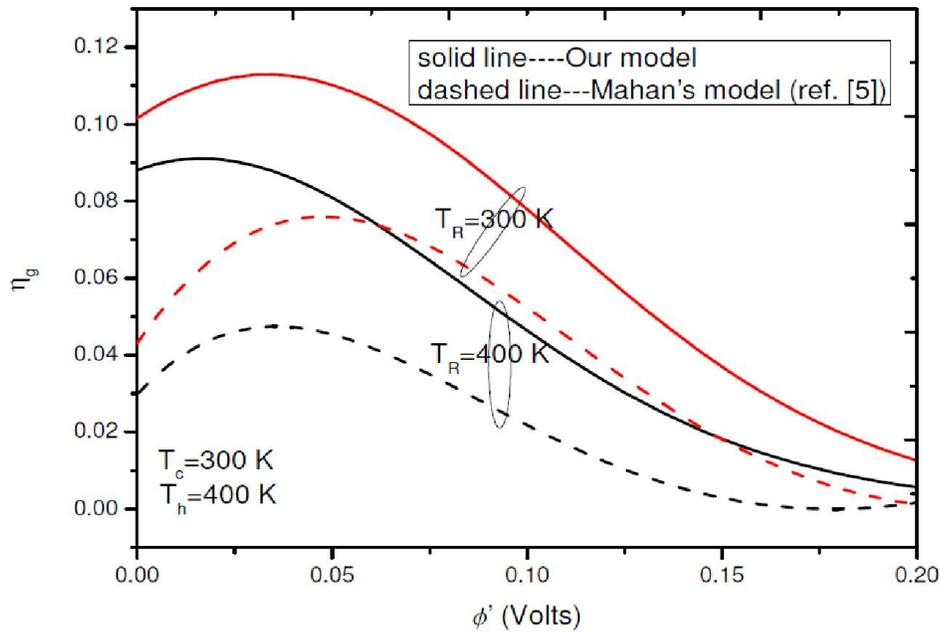
**Fig. 4:** A comparison of our model (solid lines) with Mahan's model (dashed lines - [5]) at  $T_c = 300$  K and  $T_h = 400$  K for  $T_R = 300$  K and 400 K.
