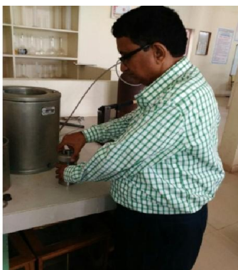
Fig. 6. Determination of Calorific value by Bomb Calorimeter
