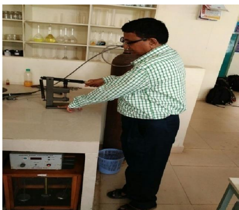
Fig. 7. Pellet Sample Making of dry MSW
