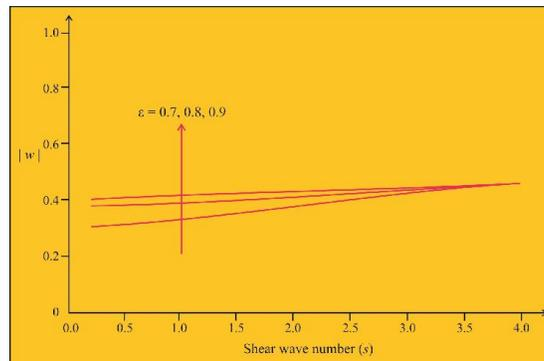
Fig. 4. Phase velocities for different values of Porosity taking  $Da = 1.0$  and  $\bar{M} = 0.3$  except for  $Da = 0$ ,  $\varepsilon = 1.0$
