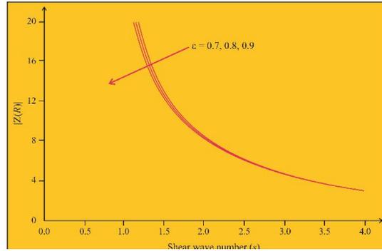
Fig. 3. Attenuation for different values of porosity taking  $Da = 1.0$  and  $\bar{M} = 0.3$  except for  $Da = 0$ ,  $\varepsilon = 1.0$
