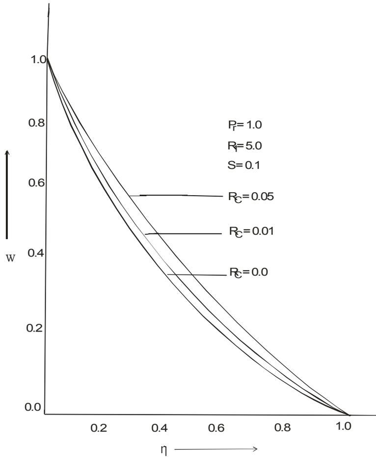
Fig. 1. Effect of  $R_c$  on velocity field.
